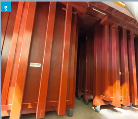
g The pre-treatment line baths seen from below. Both the baths as well as the collecting basin are completely coated with acid-proof laminate.
